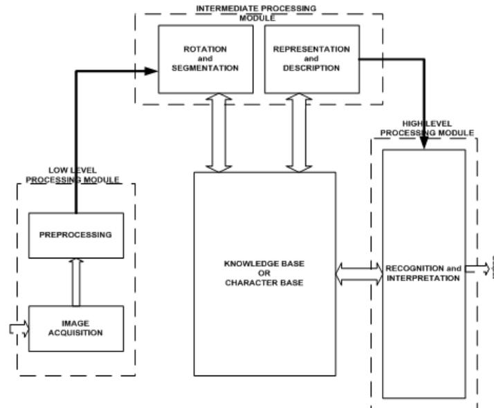
Figure 3. Schematic of the off-line Yoruba Optical Character Reader
